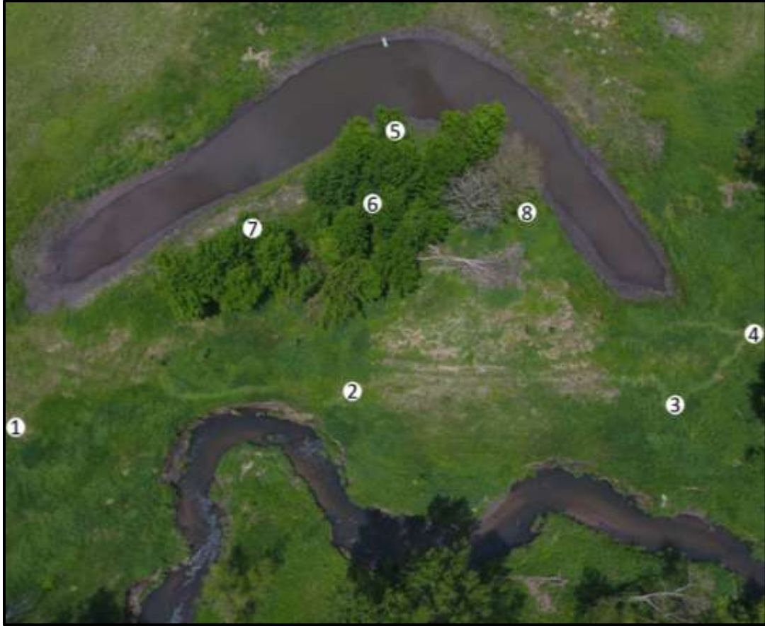
Figure 3.3. Location of eight groundwater monitoring wells installed to measure groundwater quality and hydraulic gradient. Transect 1 is composed of wells 1-4, transect 2 is wells 7-8, and transect 3 include wells 5-2.
